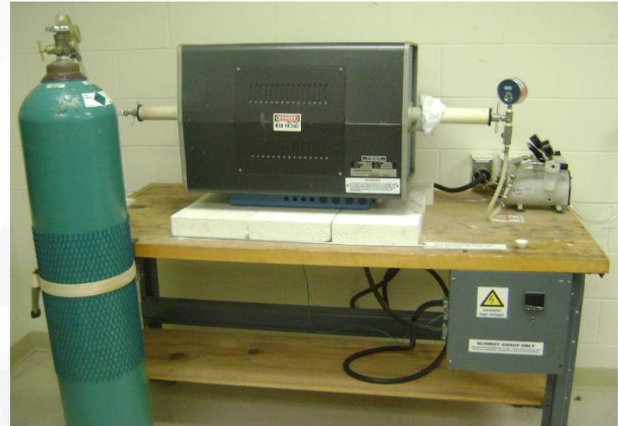
Fig. 9. CVD experimental set up for synthesis of 2D carbon nitride [3].
