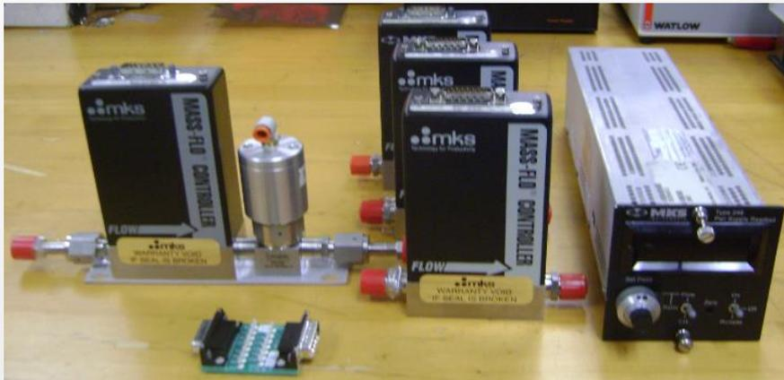
Fig. 20. Mass flow controllers, Flow meter by mks as depicted in Fig. 16, of the proposed gas delivery system .
