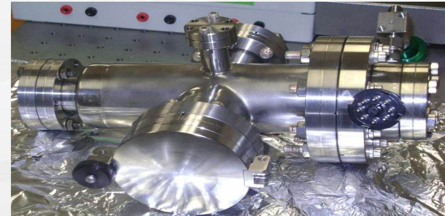
Fig. 21. Side view of the Vacuum sub-system, showing the chamber loading door and gas inlet nozzles.
