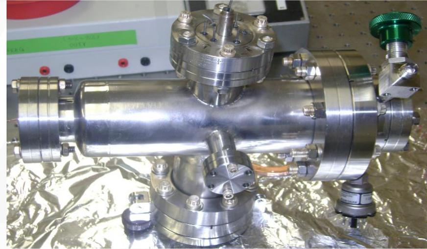
Fig. 19. Top view of the Vacuum sub-system chamber, with various connection ports, for deployment in CVD process.
